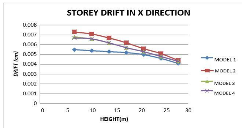
Figure 9: Storey drift in 8 storey structure in x direction
